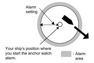
How the anchor watch alarm works
